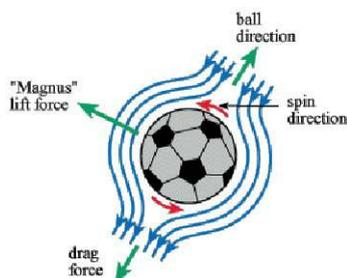
The movement is generated by the introduction of circulation through spin and using the Bernoulli effect.
