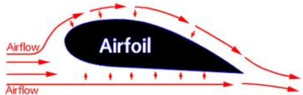
The lift is caused by the fact that the air flows faster on the upper surface of the wing compared to the lower surface.
