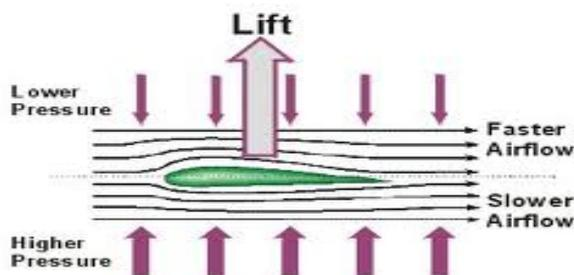
Both the shape of the aerofoil and the angle of incidence to the flow are important.
